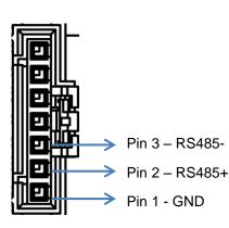
Port: JP2 Connector Type: 2.54mm Pitch Rectangular Drive Header: (Molex) 70553-0041 Plug Connector: (Molex) 50-57-9407
