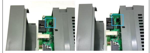
3. Inserting the jumper connects the terminating resistor. Removing the jumper disconnects the terminating resistor. By factory default, the servo drive does not have the jumper connected.
