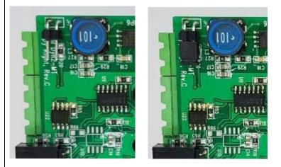
3. Inserting the jumper connects the terminating resistor. Removing the jumper disconnects the terminating resistor. By factory default, the servo drive does not have the jumper connected.
